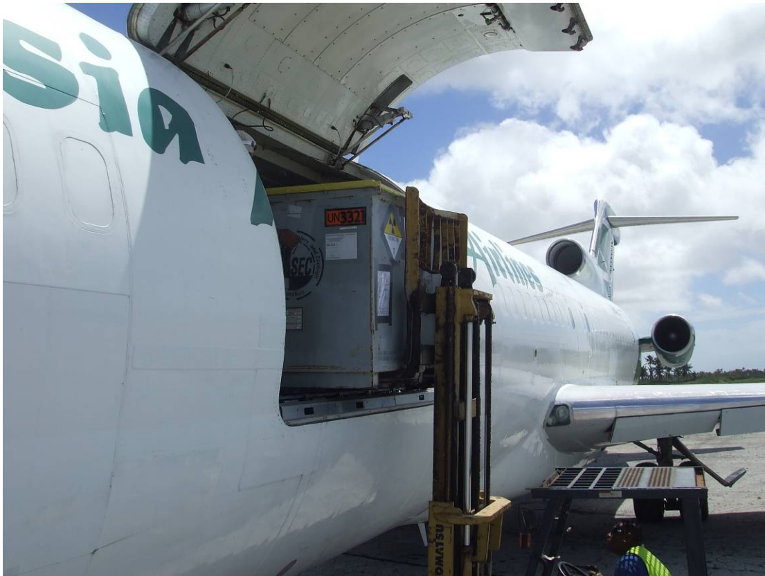
Fig. 4. Radioactive waste inside a B25 box being loaded into a cargo plane at Cassidy airport on Kiritimati Island.
