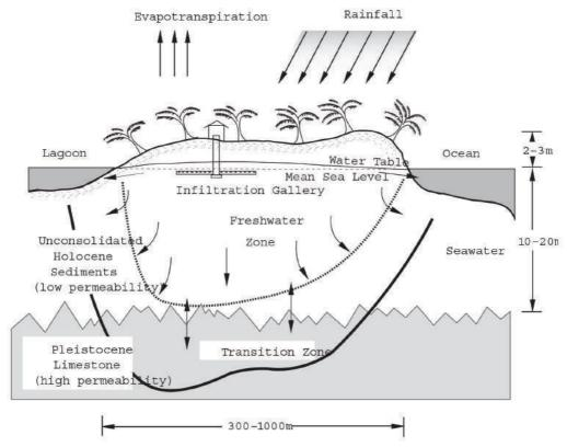
Figure 23: Cross section of an atoll freshwater lens.
