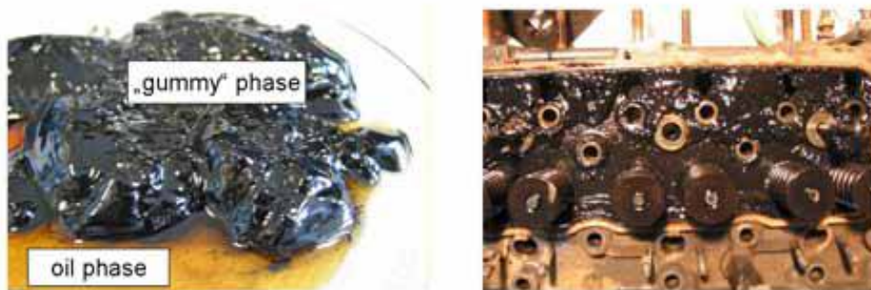
Picture 5.2: Polymerisation and Phase Separation of Engine Oil
